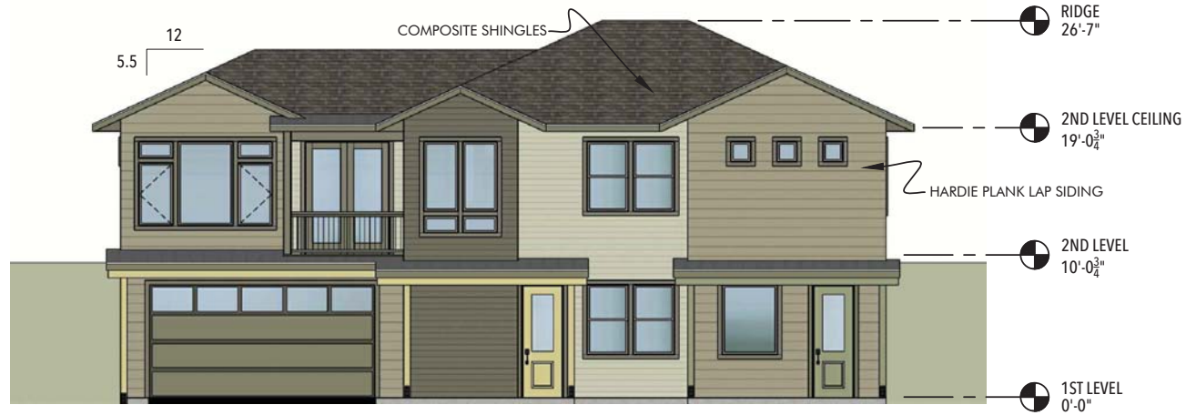
West Elevation - Facing Patton Ln.
