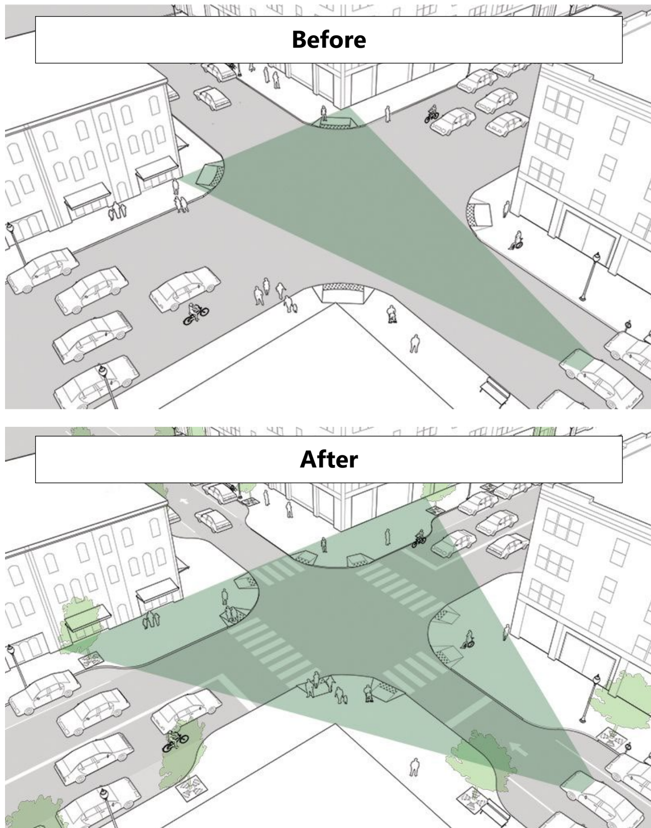
Figure 15. Curb Extension Sight Distances
