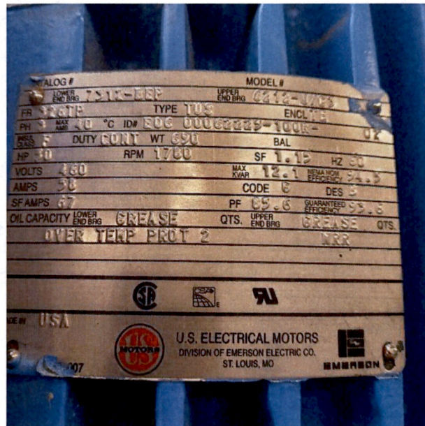
Regional BPS 50 hp pump motor tag
