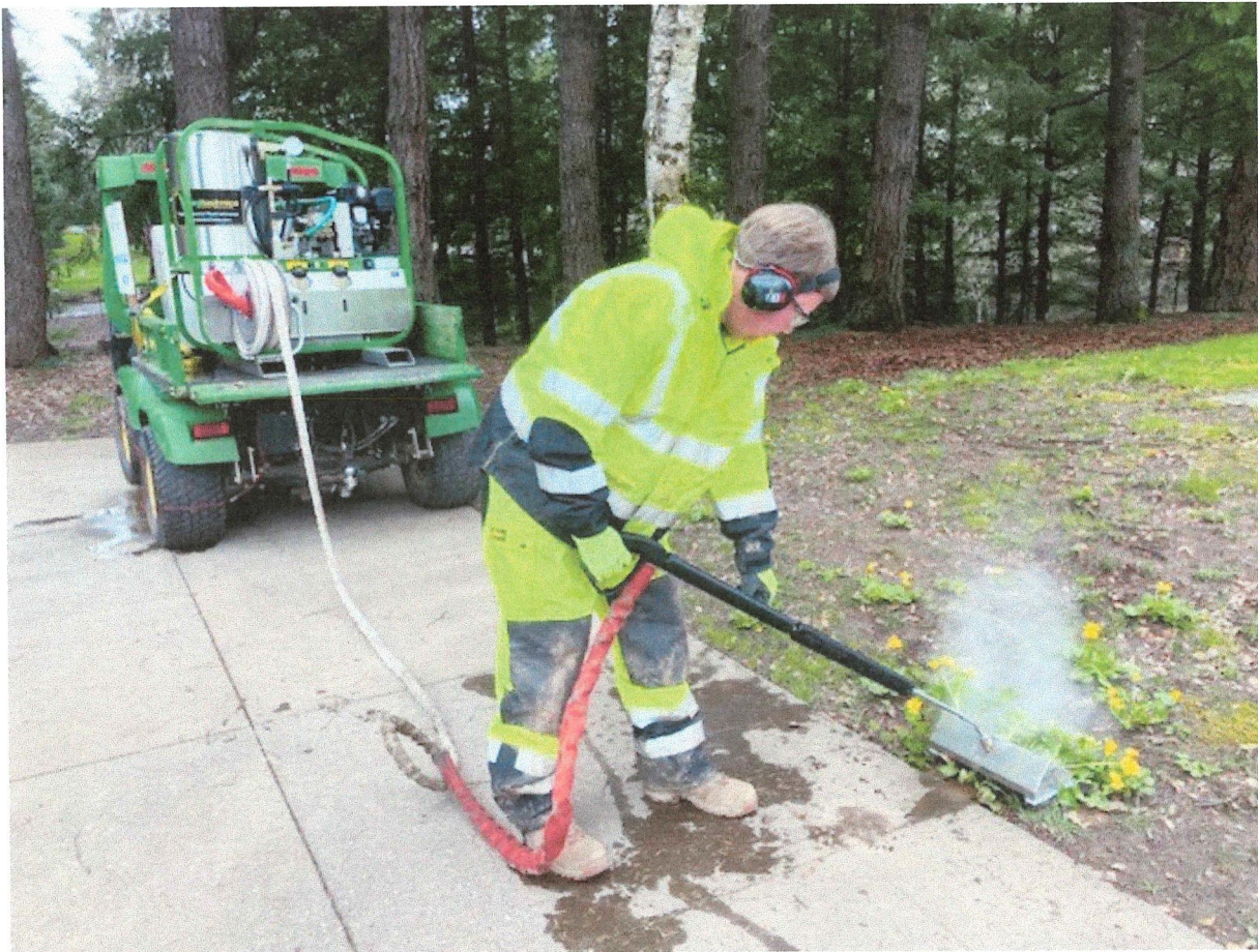
photo of Wilsonville Oregon's steam weeder in action
