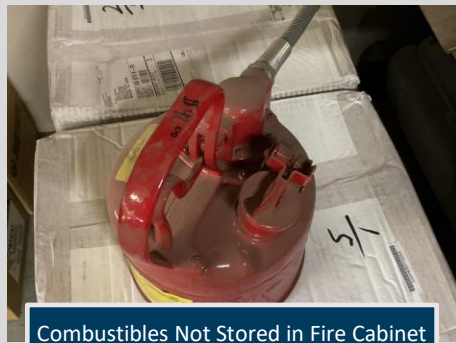
Combustibles Not Stored in Fire Cabinet
