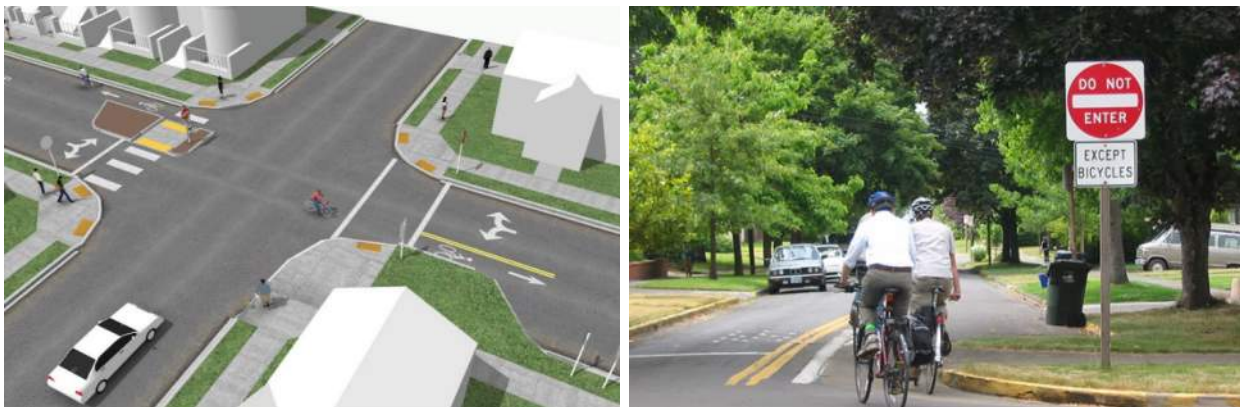
Figure 13. Traffic Diversion: Partial Closure
