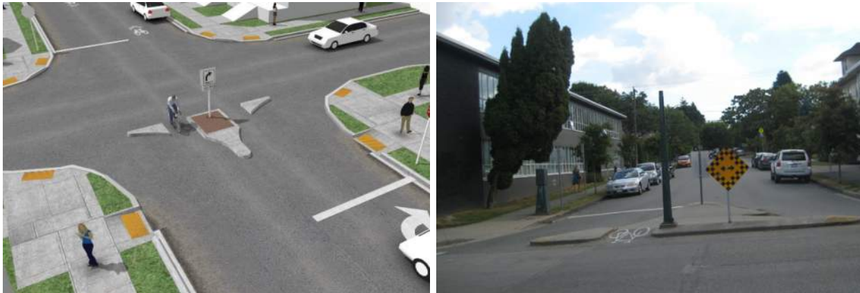
Figure 12. Traffic Diversion: Right-in Right-Out Diverter
