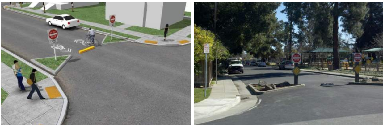
Figure 15. Traffic Diversion: Full Diverter
