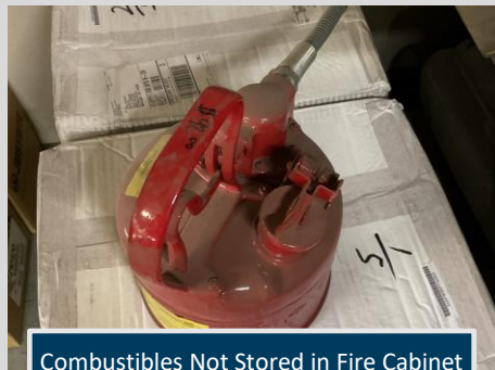
Combustibles Not Stored in Fire Cabinet
